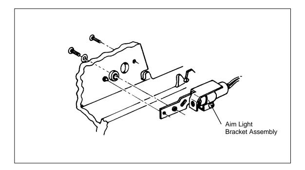
Figure 5-15 Aim Light Cable Assembly
